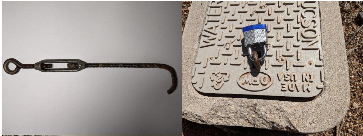
Modified turnbuckle for securing meter box lid
